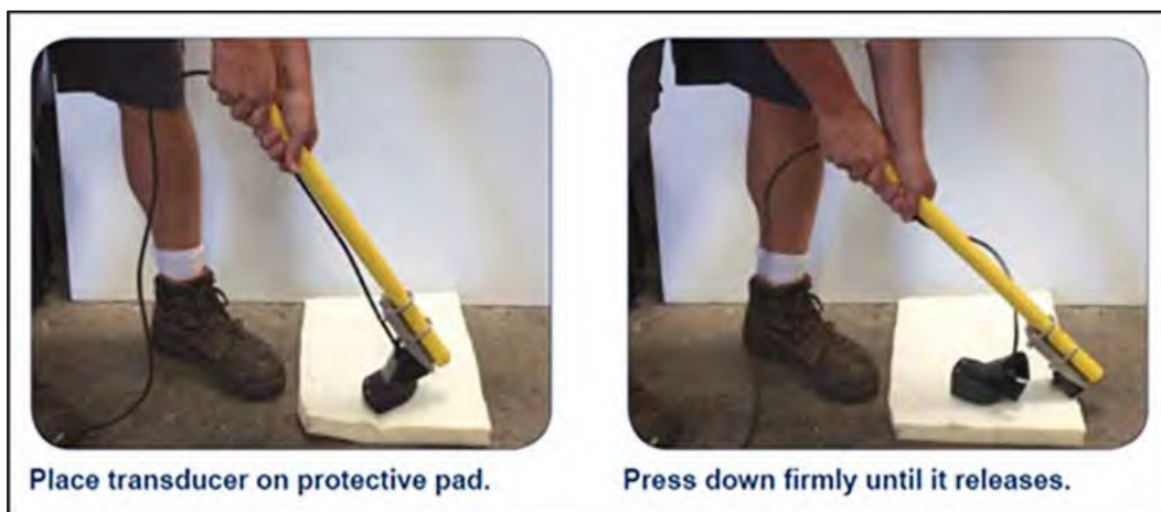
Figure 4.—Removal of transducer at completion of survey (Seafloor Systems, Inc., 2017).
