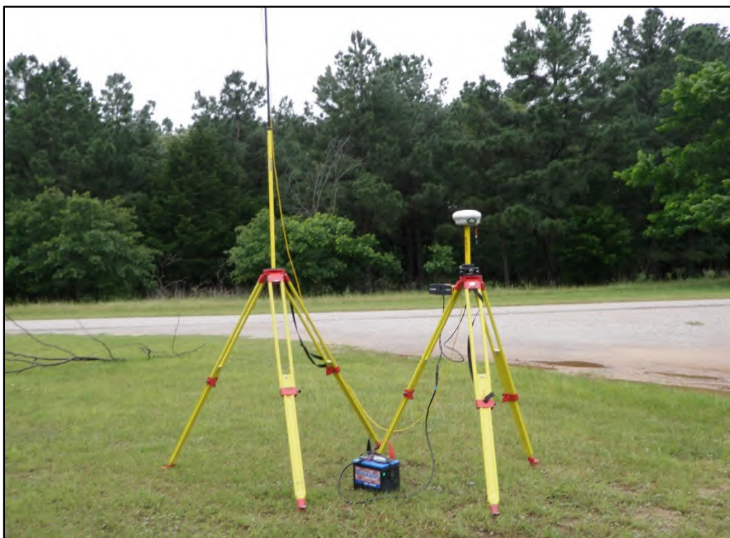
Figure 2.—Typical RTK GPS base station setup, Thunderbird Reservoir, Oklahoma.
