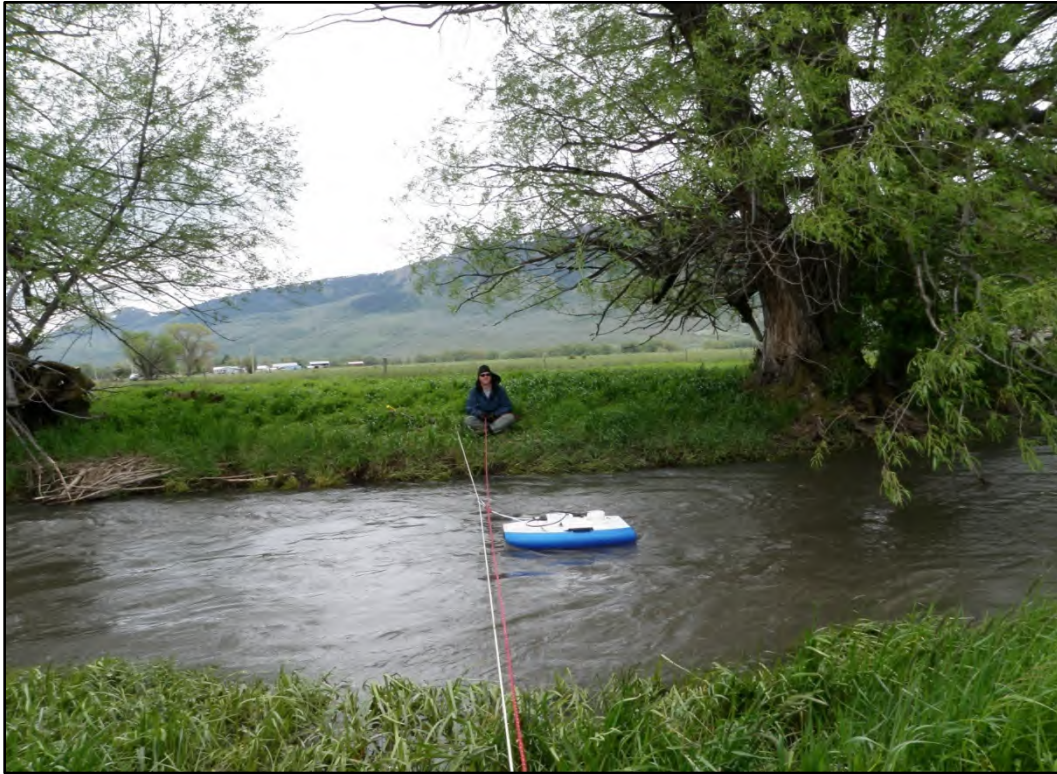
Figure 12.—Typical tagline setup with guide ropes for ferrying hydroboard back-and-forth across the channel.
