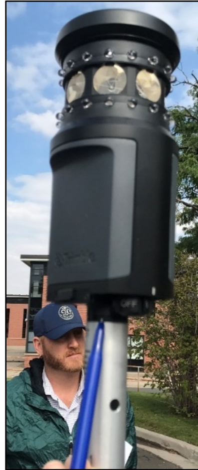
Figure 5.—Robotic prism mounted on rod. End of pen is pointing to the “bottom of mount” where rod height is measured.
