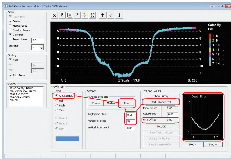
FIGURE 13. Fine Step = 0.05 sec. Increments, Number of Steps Increased to 51. This gives a more pronounced 'V' shape.
