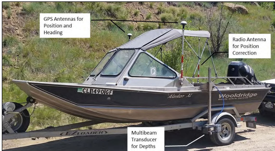
Figure 4.—Multibeam bathymetry system mounted to an SRH survey vessel.
