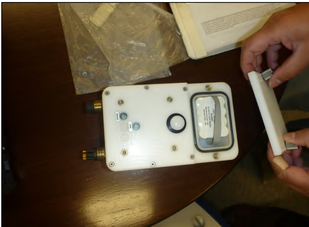
Figure 4.—Insert battery pack into power box (PCM). Verify terminals are correct.
