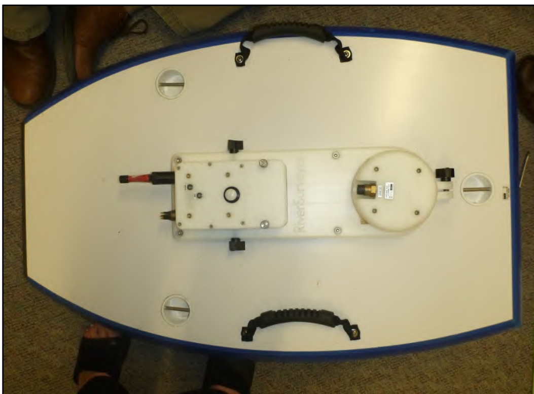
Figure 5.—Install Bluetooth antennae with red tip to power box (PCM).
