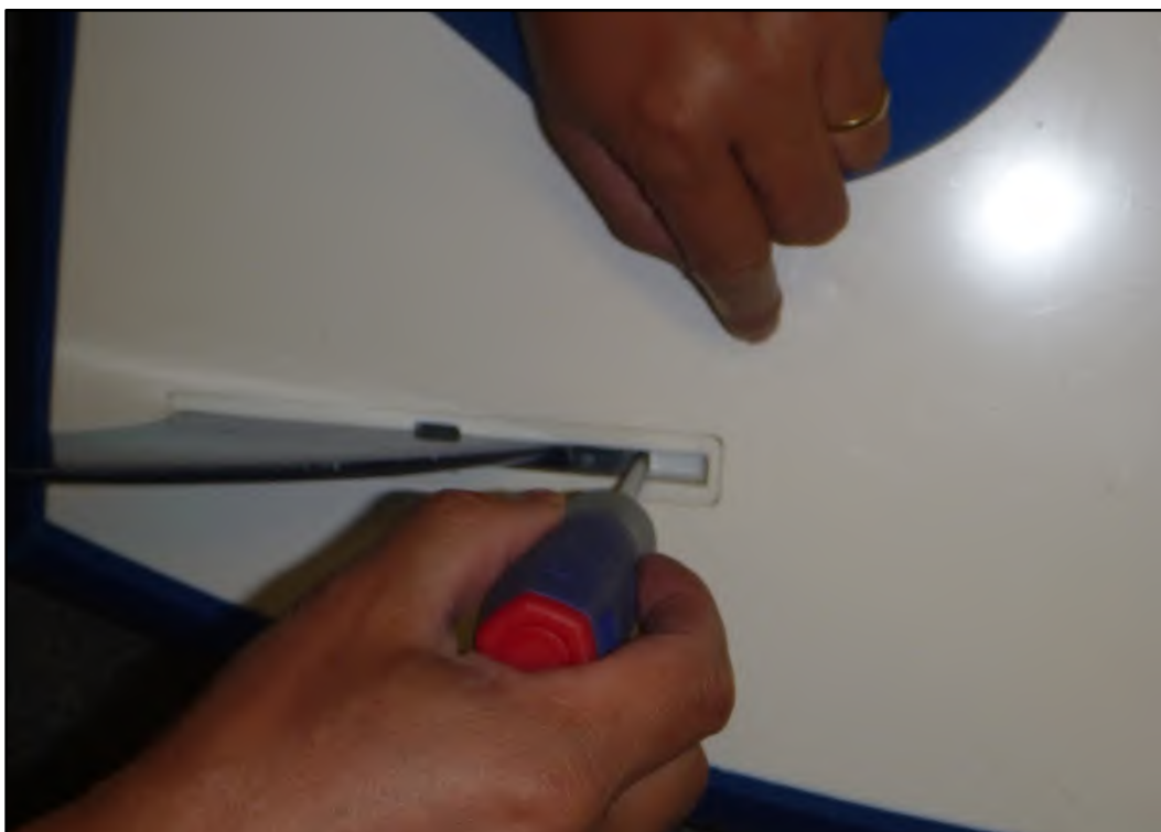
Figure 3.—Install blue fins on bottom of the ADCP by screwing fins into rectangular plates.
